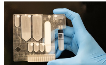
GeneCapture identifies the molecular signature of the pathogen in its 1-hour sample-to-answer cartridge.
